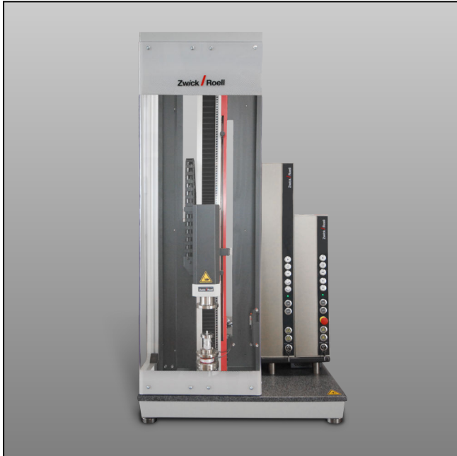
zwickiLine with torsion drive
