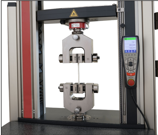
Screw Grips, Type 8355, Fmax 20 kN
